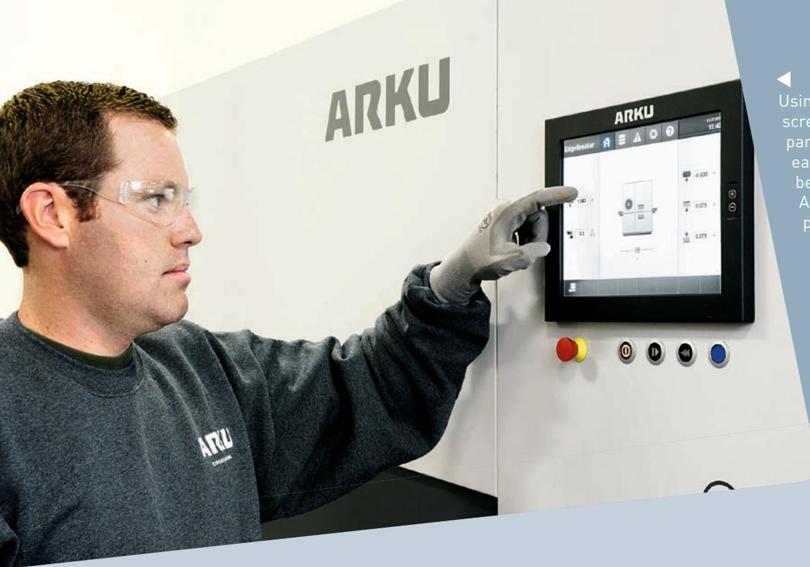
Using the EdgeBreaker® touch-screen controls, parameters for parts can be entered quickly and easily. The stored data can then be retrieved at any time. Automatic wear setting compensation is integrated.
